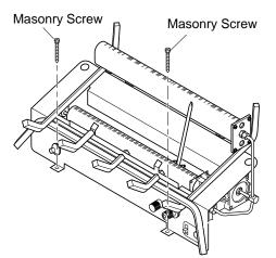
Figure 12 - Attaching Base to Fireplace Floor
